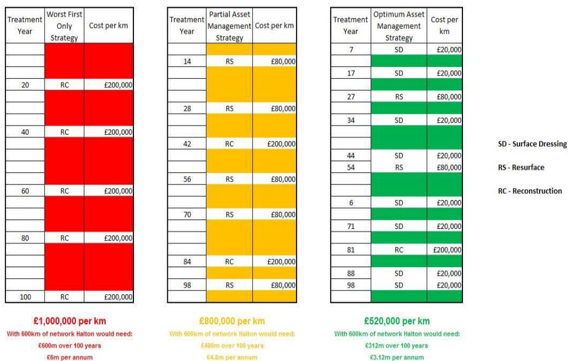
Figure 8.3 Impact of different lifecycle plans on whole-life costs per km of carriageway
